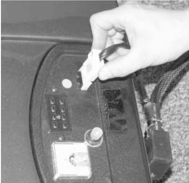
Figure 11. Charger Inhibit Connector
