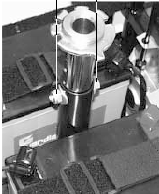
Figure 14. Seat Tower Nut And Bolt
