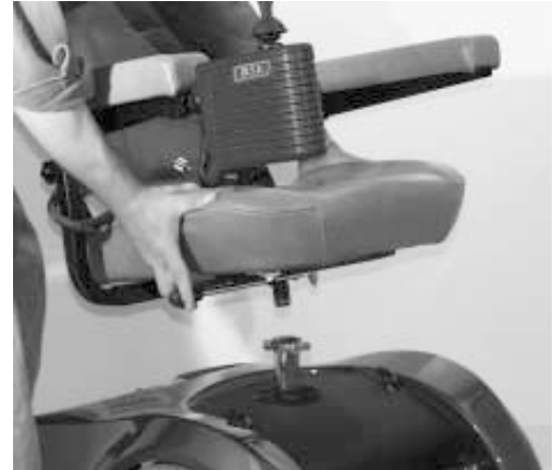
Figure 24. Removing The Seat
