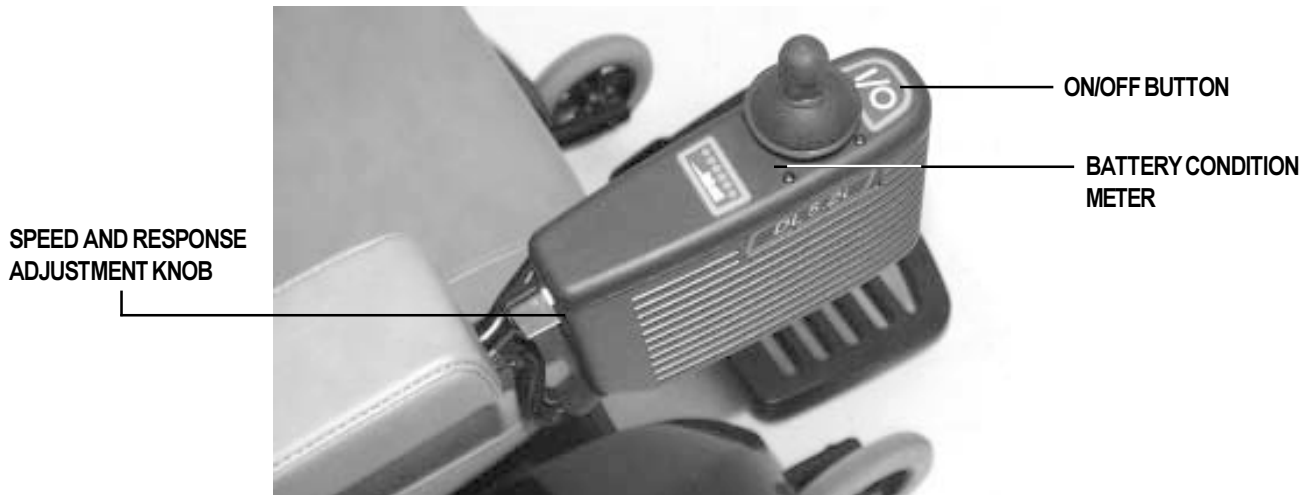
Figure 25. Dynamic Joystick Controller
