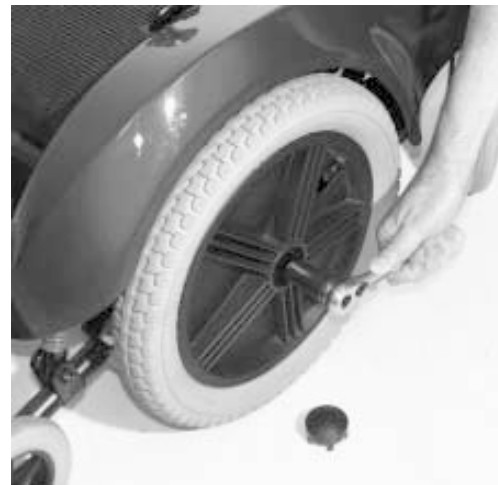
Figure 31. Drive Wheel Nut Removal
