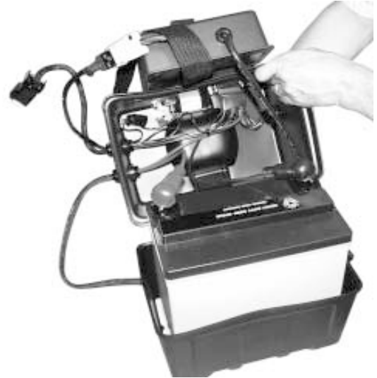
Figure 30. Opened battery box
