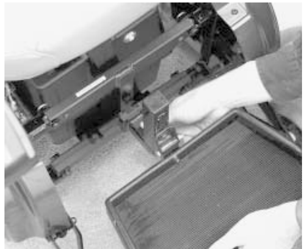
Figure 11. Mounting the footrest
