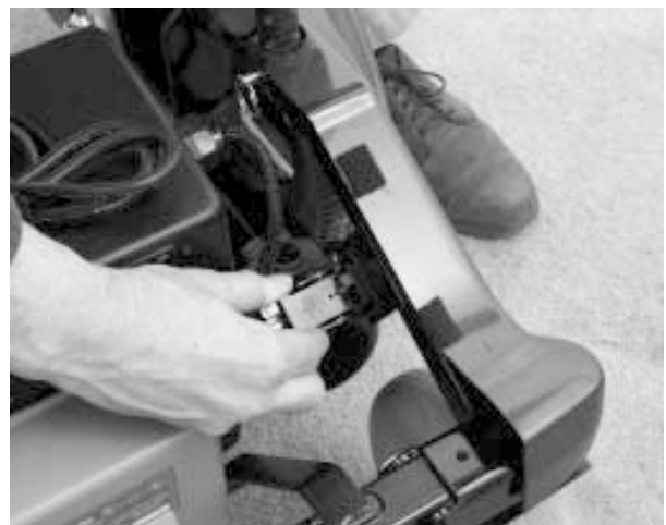
Figure 9. Motor harness connector
