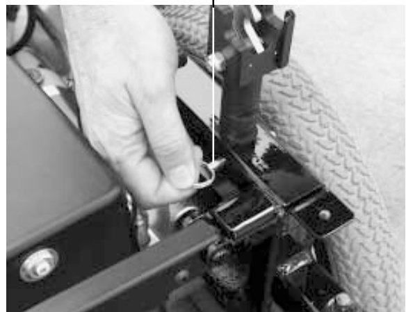
Figure 13. Seat height adjustment
