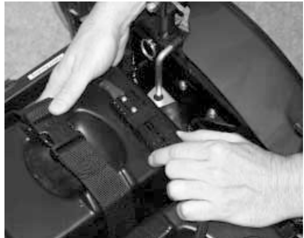
Figure 8. The front-to-rear battery cable connector
