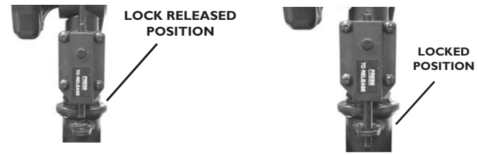
Figure 10 - Handlebar Assembly Lock
