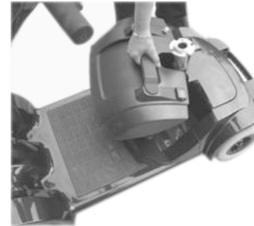
Figure 13 - Battery Case Removal
