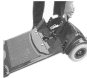
Figure 15 - Rear Drivetrain Assembly Disconnected
