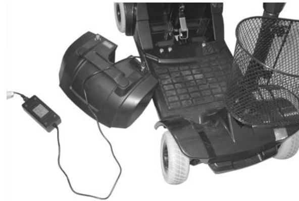
Figure 3 - Battery Charging, Off Vehicle
