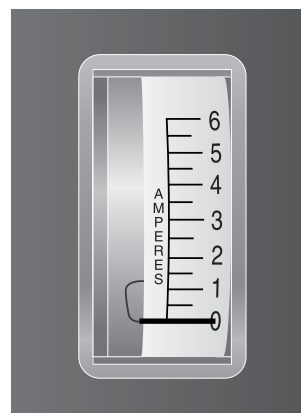
FIGURE 8. AMMETER INDICATES BATTERY IS FULLY CHARGED
