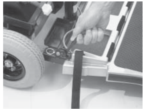
FIGURE 21. PUSH LOCKING LEVERS FORWARD
