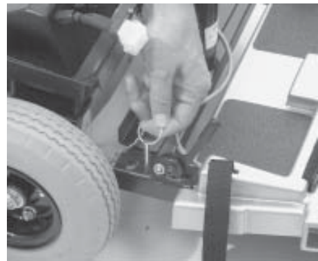
FIGURE 22. REMOVE BALL DETENT PINS WITH RINGS
