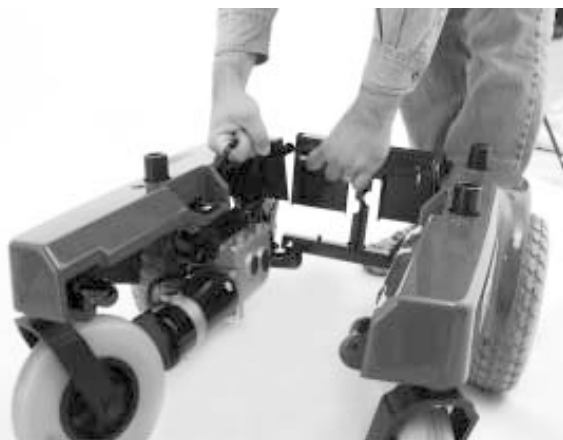
Figure 25. Fitting the Frames
