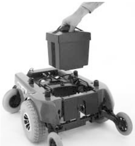
Figure 20. Removing Battery Boxes
