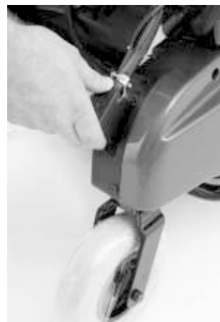
Figure 19. Plug in 9-pin controller connector.
