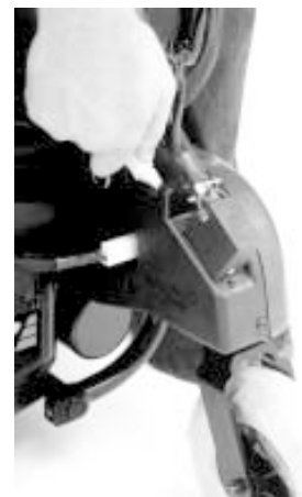
Figure 20. Plug in charger connector.
