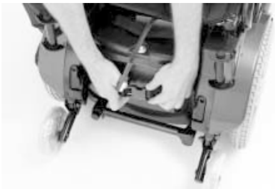
Figure 12. Install front battery box. Secure with strap.
