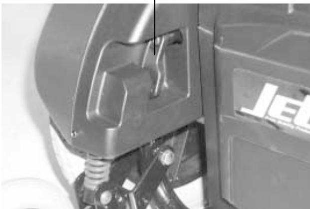
Figure 27. Drive Motors Disengaged (Freewheel Mode)
