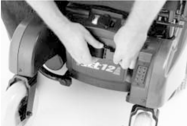
Figure 14. Install rear battery box.
