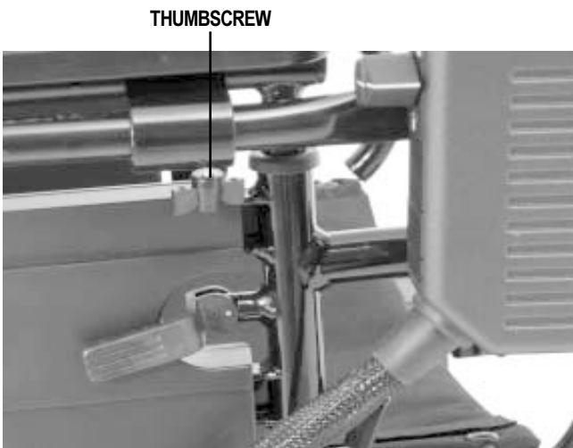
Figure 18. Install controller into armrest. Secure with thumbscrew.
