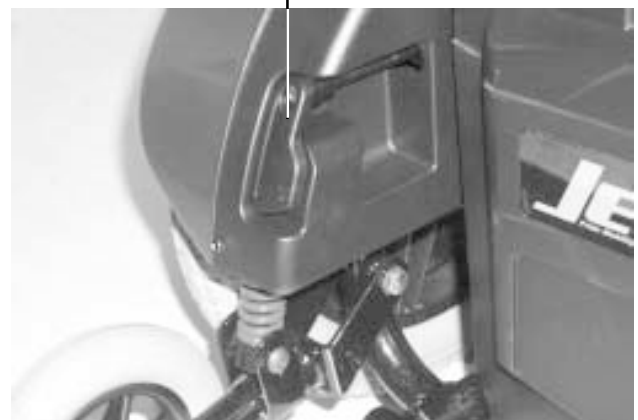
Figure 28. Drive Motors Engaged (Drive Mode)
