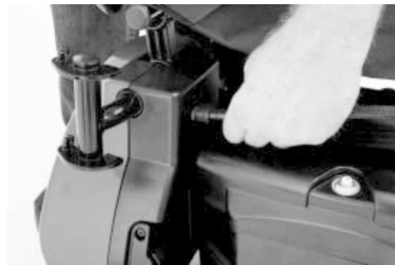
Figure 13. Connect front battery box to base.
