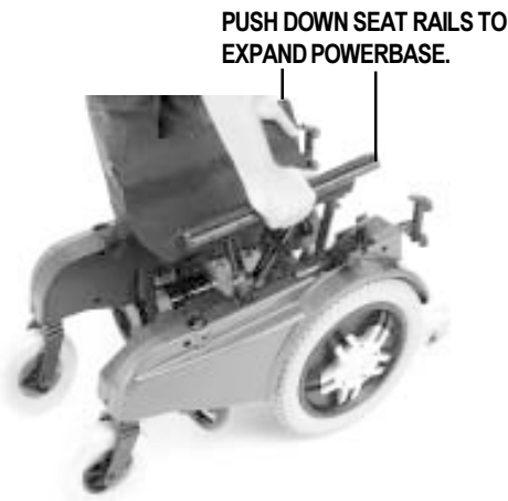
Figure 4. Press down on seat rails to open powerbase partially.
