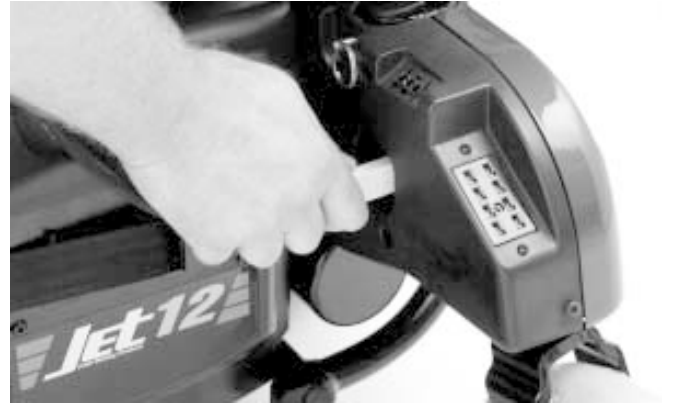
Figure 15. Connect rear battery box to frame.
