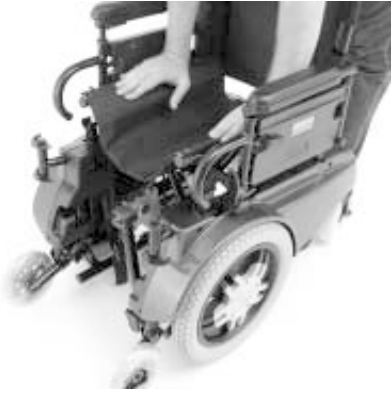
Figure 8. Press down on seat rails until they lock to expand base completely.
