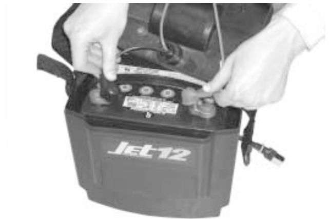
Figure 11. Install batteries into battery boxes.
