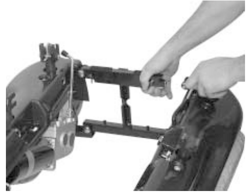
Figure 20. Fitting the Frames
