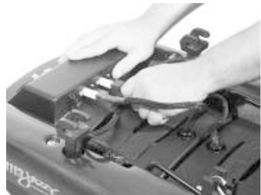
Figure 34. Disconnecting Battery Box Connections
