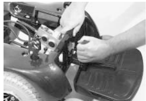
Figure 25. Mounting the Footrest
