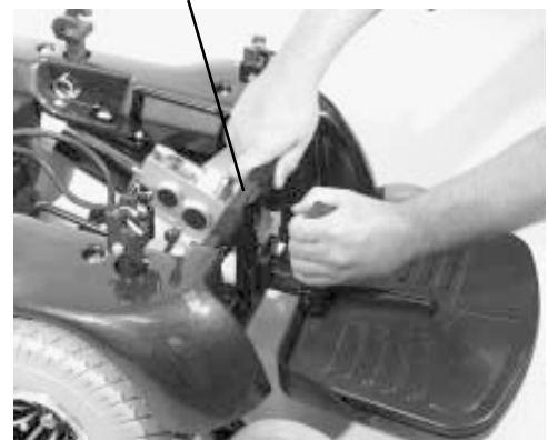
Figure 5. Remove the Footrest
