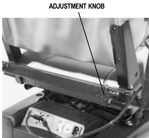
Figure 12. Armrest Width Adjustment
