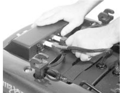
Figure 8. Disconnect Battery Cases
