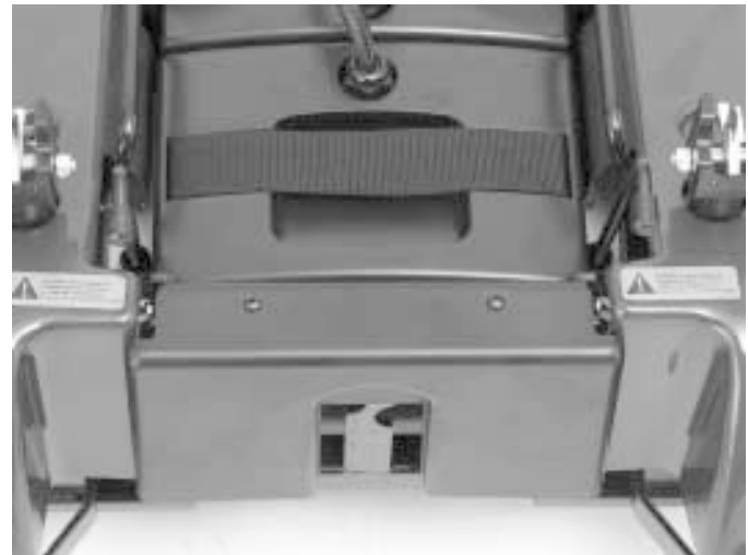
Figure 3b. Drive Motors Engaged.
