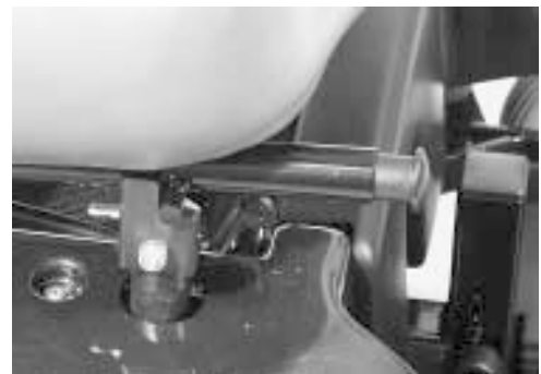
Figure 24. Locking the Seat Frame
