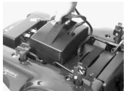
Figure 35. Battery Box Removal
