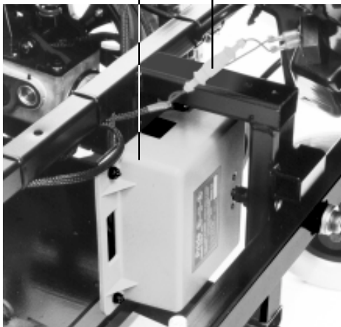
Figure 26. Onboard Battery Charger
