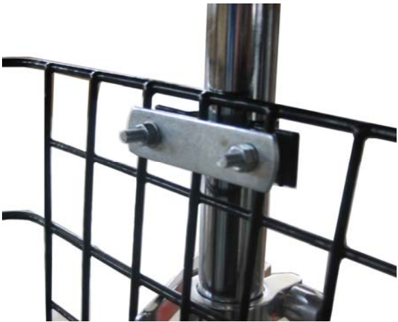
14. Screw the connecting plate and bracket together using the screws and nuts provided. (2 bolts – M5x25, 2 washers - #5, 2 nuts - #M5)
